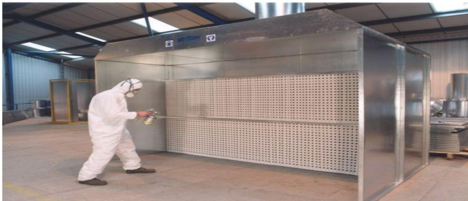
Dry back spray booth with disposable corrugated cardboard filter. (Image from airflow Ltd)
